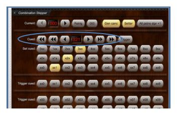
Using its arrow buttons, adjust the stepper editor's block size to the desired value, i.e. 3 in this example:
